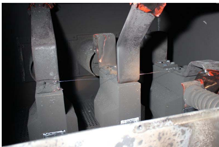
Photo 34: Test object before Test No. 114 0826 (ignition wire)
