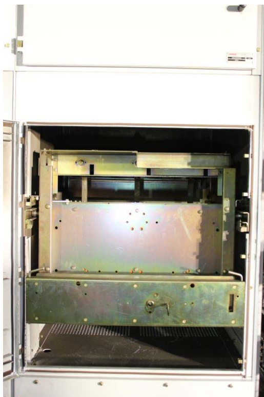
Photo 11: Test object before Test No. 114 0822 (point of arc initiation)
