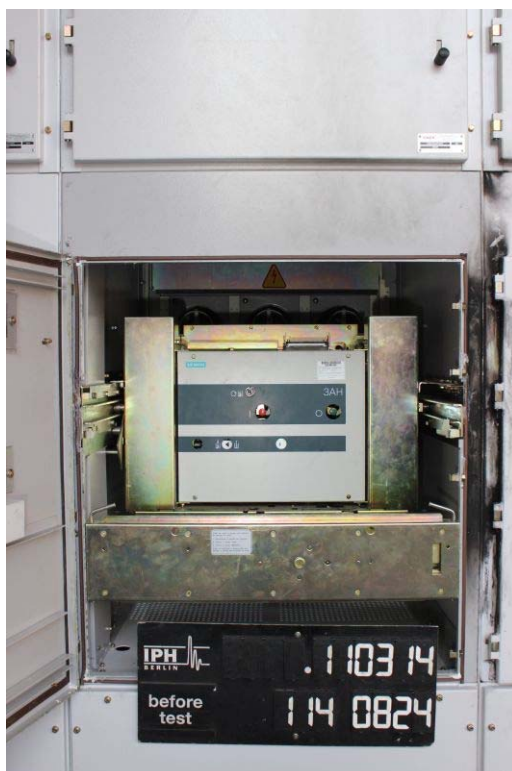
Photo 27: Test object before Test No. 114 0824 (point of arc ignition)
