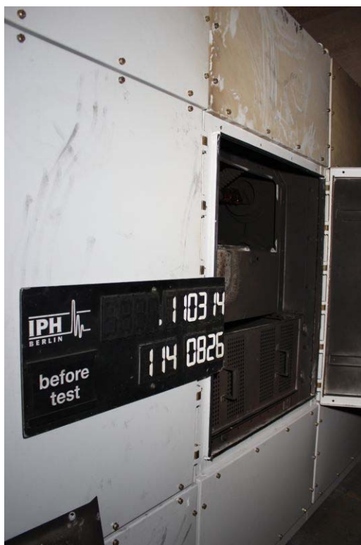
Photo 35: Test object before Test No. 114 0826 (point of arc ignition)
