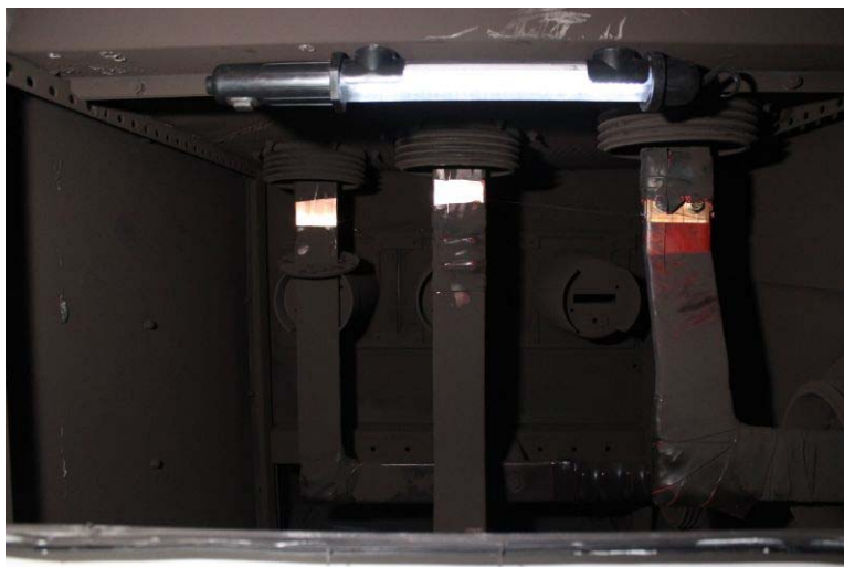
Photo 19: Test object before Test No. 114 0823 (point of arc initiation)
