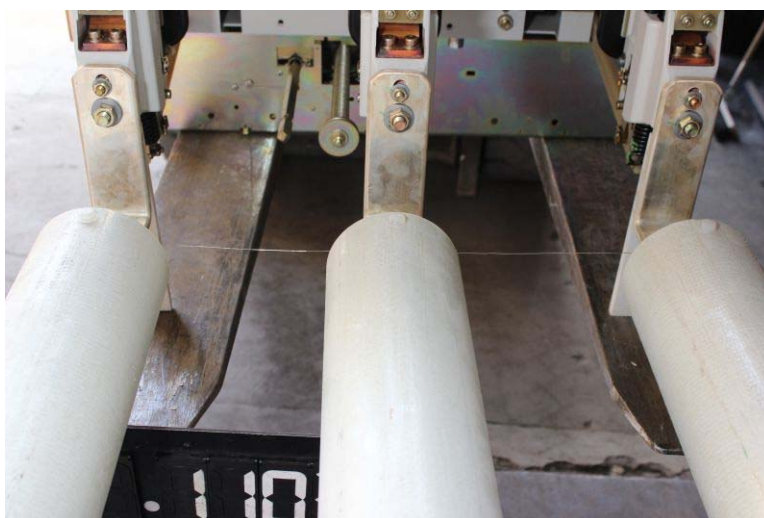
Photo 26: Test object before Test No. 114 0824 (ignition wire)
